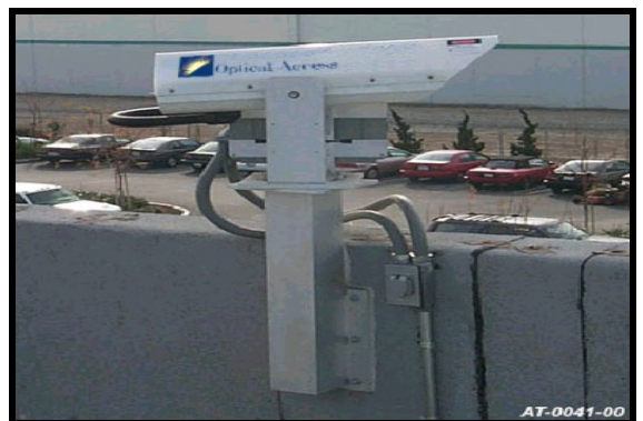
Figure 2.9: Wall Pedestal Mounting (using JMP and M054C)
